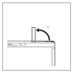
To improve the UMTS reception, swing out the UMTS antenna in the direction of the arrow (1).
